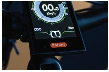
**ODO:** Odometer will display the total kilometers the bike has travelled. This cannot be reset.
